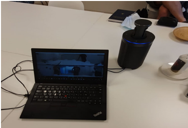
Hi-tech 360° camera that constantly films the whole room but only shows the part where someone is speaking
