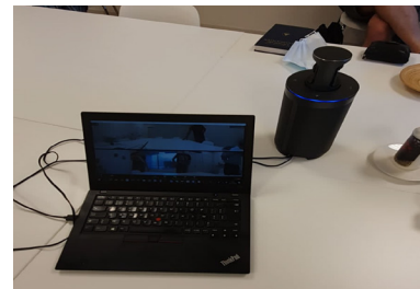
Hi-tech 360° camera that constantly films the whole room but only shows the part where someone is speaking
